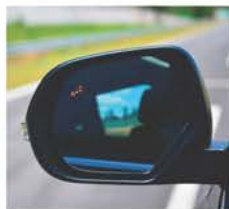
Blind Spot Warning (BSW) system (GT)
