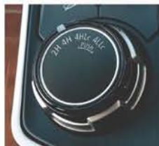
Super Select 4WD-II (4x4 variants) with Offroad Mode (GT)
